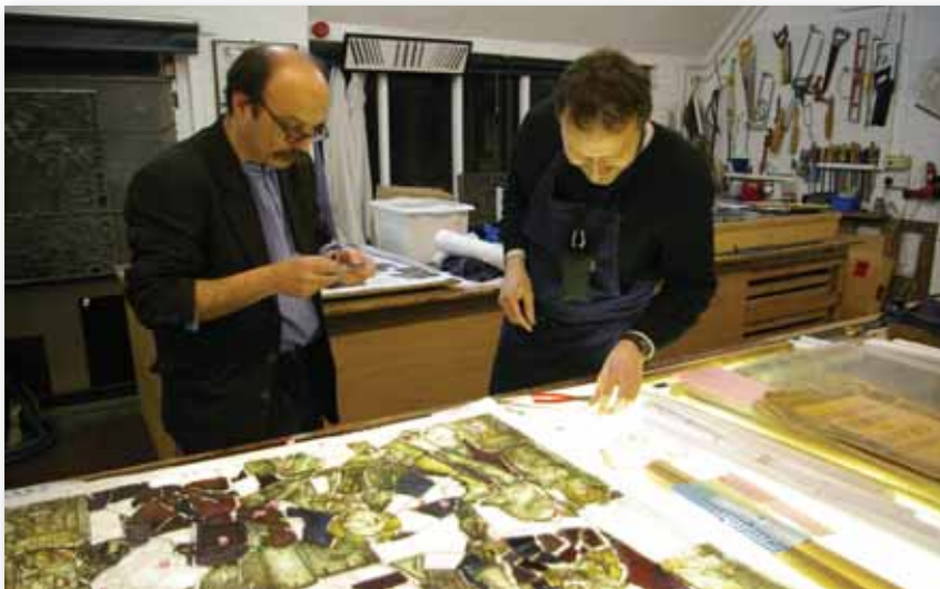
Taking samples of medieval stained glass from a panel of the Great East Window, York Minster, in the conservation studio of York Glaziers Trust.
