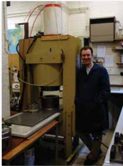
Dr de Ronde and the 1000 tonne press that he uses to apply pressure and temperature to rock samples to reproduce conditions deep in the Earth's crust.
