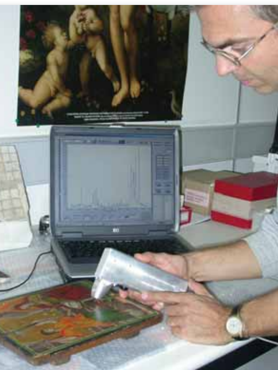
Non-destructive analysis of an icon using laser induced breakdown spectroscopy.
