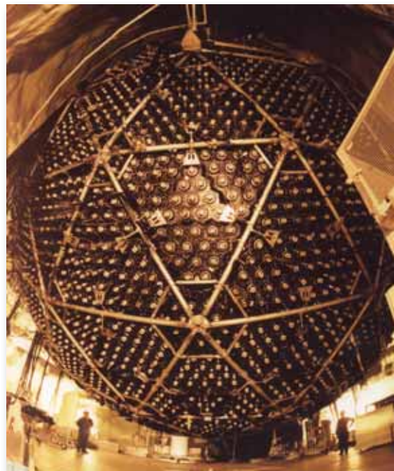
Located 2km down a Canadian nickel mine the SNO+ detector is a huge sphere of liquid scintillator which emits a flash of light when particles interact in it. The amount of light, detected by thousands of ultra-sensitive light sensors, tells us the energy of each interaction.
