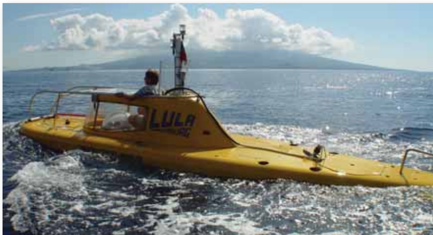
LULA the manned submersible used to research the deep (cold) water corals growing at a depth of between 200 and 500m around the Azores archipelago. Images courtesy of Rebikoff-Niggeler Foundation.
